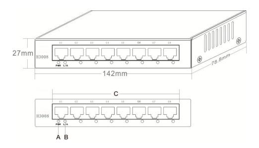
A. PWR Led Indicator B. LINK/ACT Led Indicator C.5\*10/100/1000M RJ45 Ports
